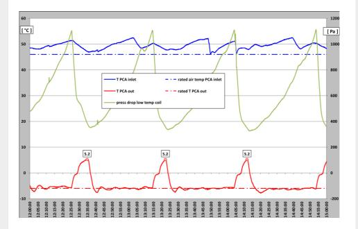
Under rated conditions the ISTinox PCA unit produces the required air flow rate (15'000 kg/hr) and cools it constantly to the required temperature. In order to optimize the cooling of the aircrafts, the new DXi unit has two cooling coils to ensure continuous cooling of the aircraft even during defrosting. In addition, the new refrigeration concept also optimizes the regulation of the defrost cycle.
