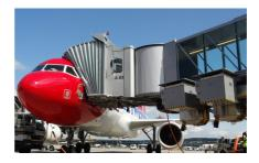
De-icing only takes place when it is necessary and, contrary to existing systems, it is not timed but measured. The de-icing cycle takes place approximately every 50 minutes and lasts around 6-8 minutes. During the defrosting cycle, the first compressor runs continuously; thus, the temperature of the PCA does not climb to values higher approx. 5,5°C during the defrosting cycle and continuous cooling of the aircraft is guaranteed.
